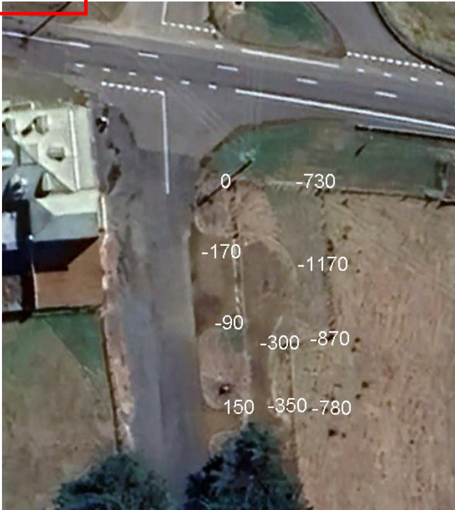
Current RL's (left – white lettering) and proposed mm ground level build-up (right – green lettering).
