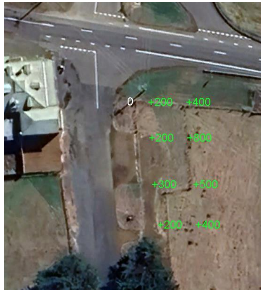
Current RL's (left – white lettering) and proposed mm ground level build-up (right – green lettering).
