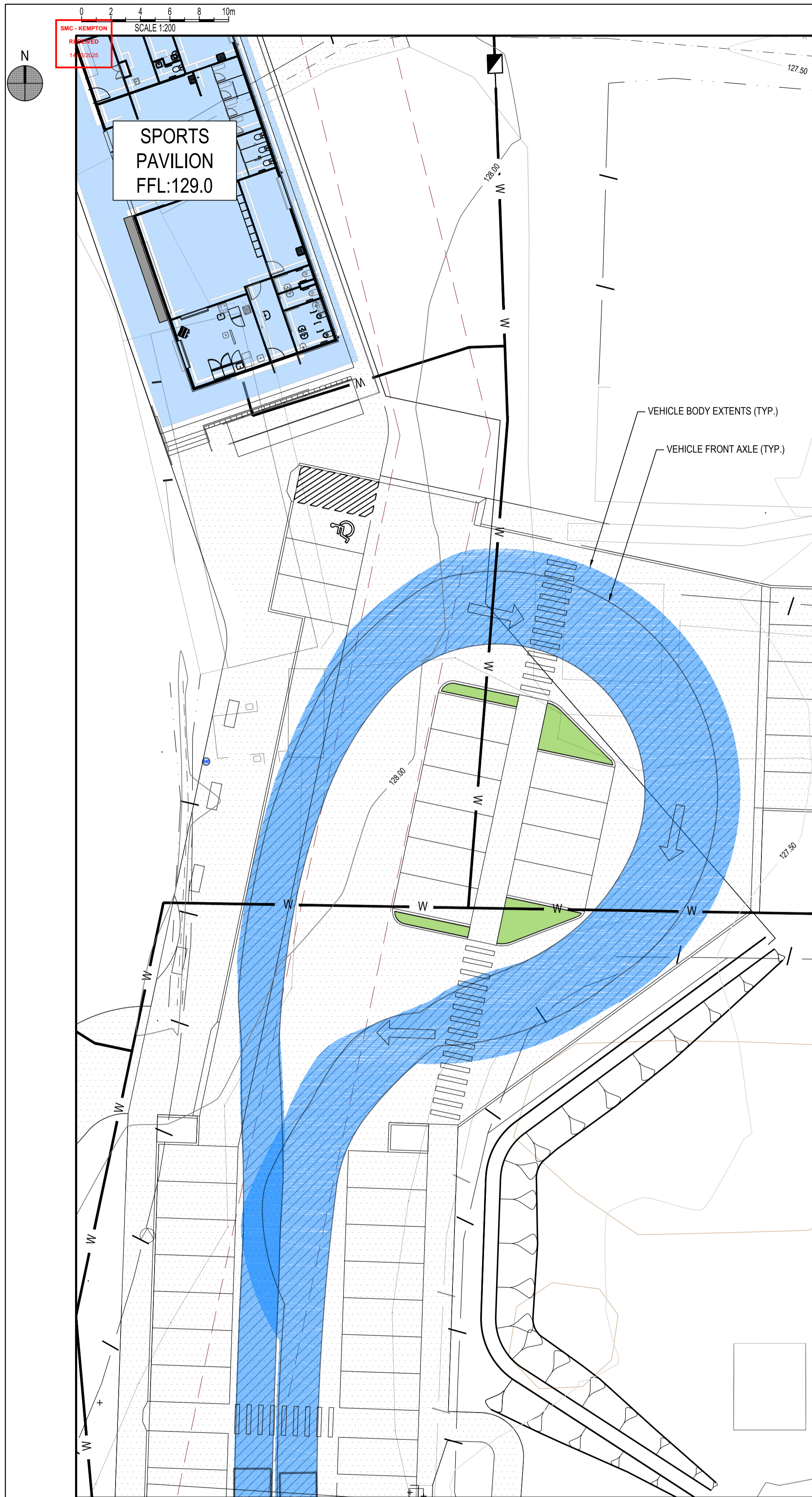
14.5m BUS TURNPATH INTERNAL MANOEUVRE
