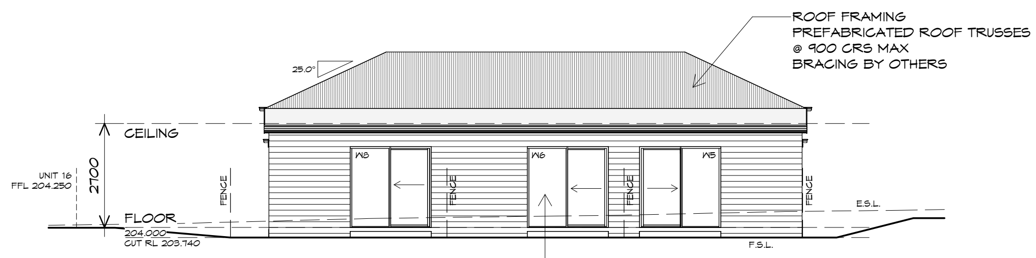
NORTH EASTERN ELEVATION 1 : 100
